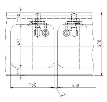
Overflow is a standard equipment of the tables with sinks.
